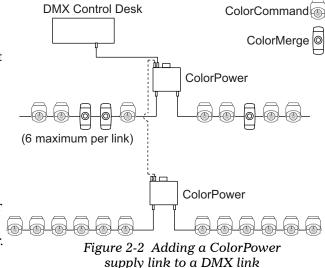
After connecting the ColorPower supply link, you will need to address the ColorPower supply and the attached fixtures/modules for identification by the DMX controller. A fixture on a DMX link is addressed by assigning it a Start Channel from 1-512. Start channels are set in the ColorPower menu system. You can choose
