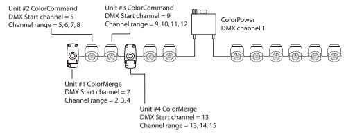
Figure 2-5 Sample automatic assignment of DMX start channels
