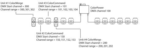
Figure 2-4 Sample manual assignment of DMX start channels
