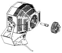
Figure B-1 Removing the lamp
