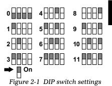
You can choose any order for fixtures on a link and any DIP switch setting for a fixture, as long as each fixture in the link is assigned a unique unit address.
