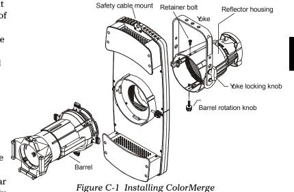
2. Insert the ColorMerge module into the Source Four rear housing assembly by aligning the mounting tabs into the rear-locking ring of the ColorMerge module. You must rotate the ColorMerge module until the Source Four mounting tabs are captured in the ColorMerge locking ring channels.
